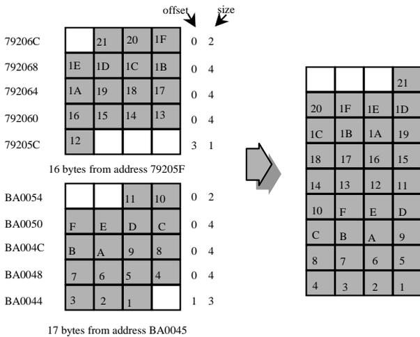
Figure 7. Word Alignment Circuit's Input and Output
