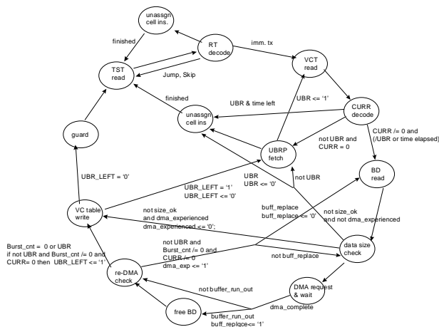
Figure 3. Simplified State diagram of the main segmentation manager
